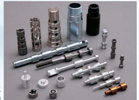
複雑・高精度研削加工 Grinding of complex and highly precise shapes
