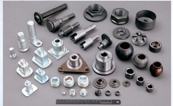
複雑、精密冷間鍛造加工 Cold forging components of complex and precise shapes
